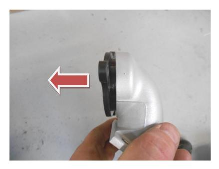
6. Lubricate the internal O-ring inside the cast elbow.
