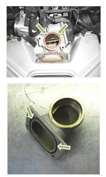
8. Ensure the O-rings in both the cast elbow and bypass valve are seated correctly.
