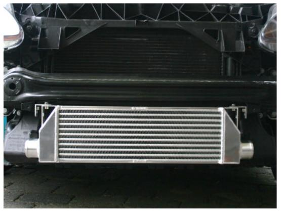
6/ Remove the oil seals from the original intercooler hoses and fit these to the corresponding new aluminium hose couplings as pictured below. Fit the hose couplings into the respective fittings on the original intercooler and the turbo outlet pipe on the right side running alongside the engine sump. Make sure the spring clips are located securely to prevent these couplings from being blown out of the fixings under boost.
