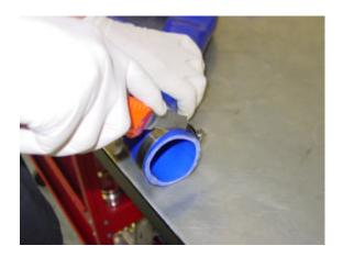
8/ Now centralise and tighten the fixing bolts on the intercooler. Fit the ambient temperature sensor by using two plastic strips as indicated below.
