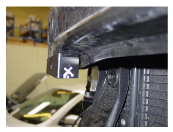
5/ Attach the brackets to the crash bar as pictured below using the nuts and bolts supplied. Then mount the intercooler into place also but only assemble the fixing nuts and bolts loosely at this stage.
