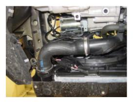
3/ Remove the horns from their brackets, now remove each bracket from the car and refit the horns as per the pictures below with the new brackets supplied so they are now sited higher. This is to allow the new hoses a free routing below the horns.
