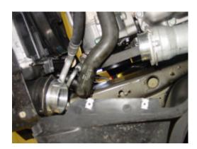
7/ Now fit the new hoses to join all the couplings and the new intercooler. The hoses require a test fit to make sure they do not foul on any other engine or front panel components. A small amount of trimming is required on the hoses at the new intercooler joints. Once you are satisfied with the fitment then secure all the hoses with the hose clips supplied.
