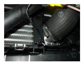
The Original intercooler can now be removed. It may be easier, when stood at the front of the vehicle to remove your right hand side first before removing your left hand side. Now install the aluminium bobbins provided over the existing intercooler mounts. These simply provide a larger mounting surface area to mount to.
