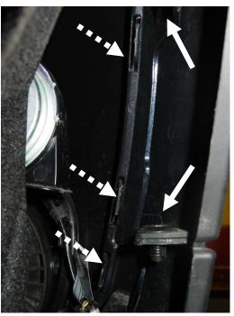
With the fasteners removed the wheel arch liner can be pulled away. The outer wheel arch trim is secured by two of the pushpin type fasteners that require removal and three plastic tabs (dotted arrow) These can be "released" by pushing with a flat blade screw driver.
