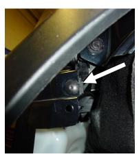
With the wheel arch trim loose at the front it is possible to access and remove the T25 Torx screw that secures the front panel.
