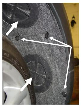
The next fasteners to be removed are those that secure the wheel arch liner at the front. With the vehicle suitably supported, and the front wheels removed it will be easier to gain access to these. Also remove the two round access covers by rotating and withdrawing.
