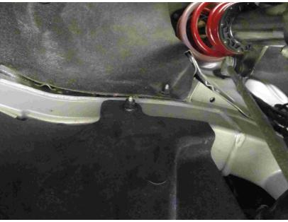
You will now need to pull back the fabric portion of the fender liner to expose the 2 nuts securing the bumper to the fenders. Remove these.
