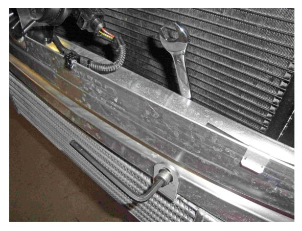
With the core now fitted, you will install the supplied silicone hoses to join together all of the intercooler and piping connections. The aluminium supports underneath the car, while obtrusive, should not prevent fitment of the hoses.
