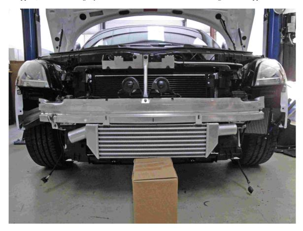
With the markings in place for the core mounting tabs, remove the core and use your power drill and 8.5mm drill bit to drill holes through the bumper support at these two markings. The support is hollow, so holes will need to be drilled through both the forward and rearward walls of the support. Please exercise caution to ensure that the drill bit does not extend so far out of the bit holder so as not to damage the AC condenser when the rear wall of the bumper support is punctured.
