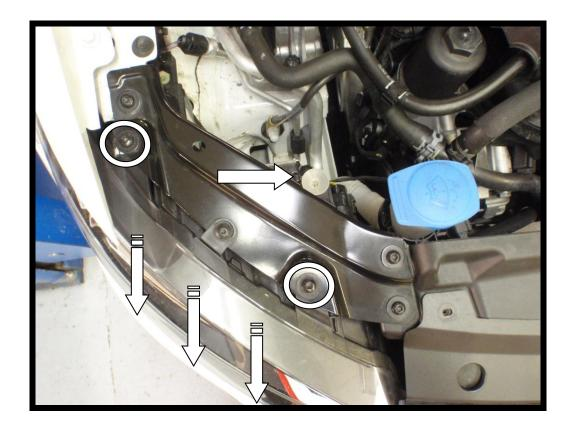
5. Undo the remaining t30 torx and flip over the plate, you will see the bonnet release mechanism. Remove the cover, pull out the cable and unhook the ball from the socket. The opposite side will just need to be removed.
