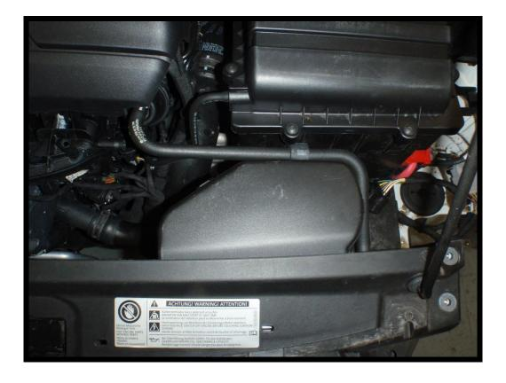
16. Undo one bolt either side of the crash bar and screw in the long bolts supplied in the kit. Remove the remaining bolts and the two t30 torx. This enables you to pull the radiator pack forward without it dropping to the floor.
