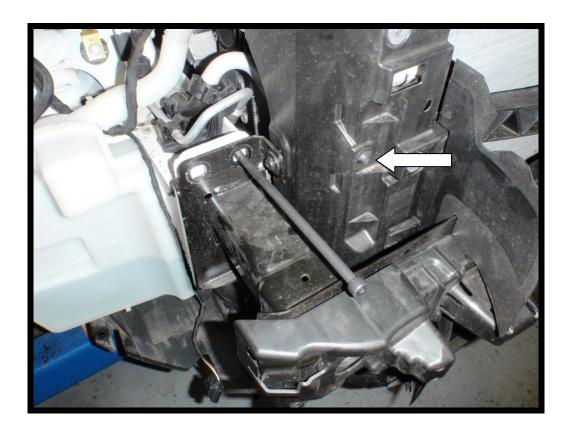
17. Using the large zip ties supplied in the kit attach the fan cowling and radiators to the lifting eyes of the engine.
