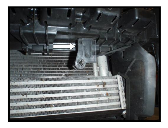
15. Remove the cooled air feed to the filter and the engine cover.
