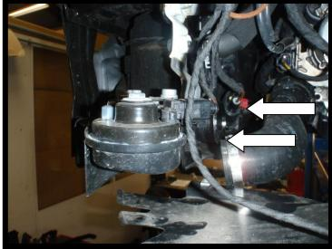
14. Unclip the temperature sensor and bracket.
