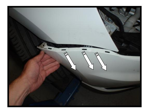
8. With an even pressure pull the bumper forwards, using a screw driver lift the two clips to release. Still applying pressure forwards push the clip behind the grill down to release, do this on both sides.
