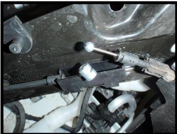
6. Undo the two t25 torx from the slam panel.
