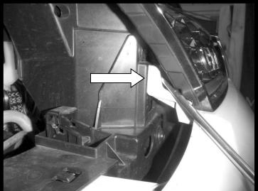
9. The slam panel has four clips that need to be pushed down and the bumper can be pulled forward. The headlamp washer hose will need to be disconnected, undo the wiring loom clips from both spot lights and remove the bumper.
