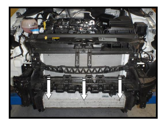
19. Unclip the OEM intercooler on the right hand bracket and remove.
