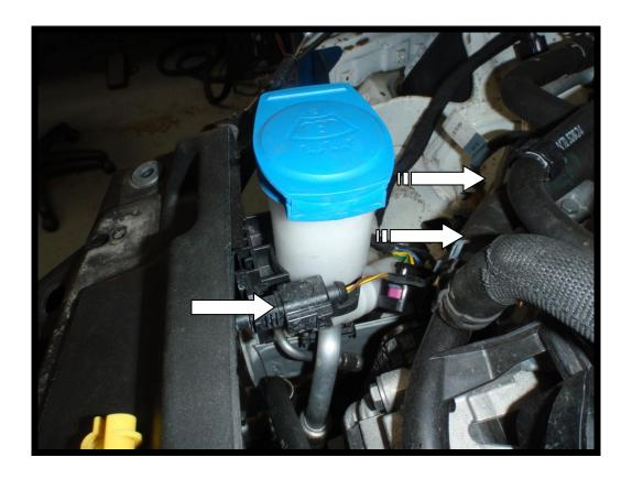
13. Unclip the wiring from the thermostat on the radiator and unclip the wiring from the horns.
