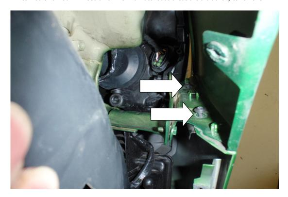
6. Now remove the T25 Torx screws under the bonnet on the front scuttle panel .
