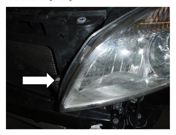
10. Remove the 10 mm bolt on each light located here on the inner wing.
