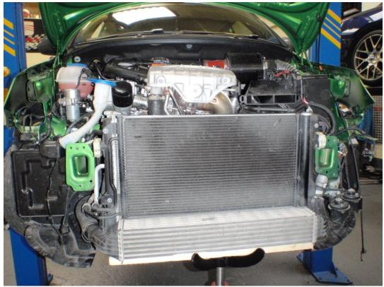
17. Using a flat headed screwdriver, unclip the bracket on the right hand side of the intercooler, then use the screwdriver as a lever and push the intercooler down off the edge of the radiator.
