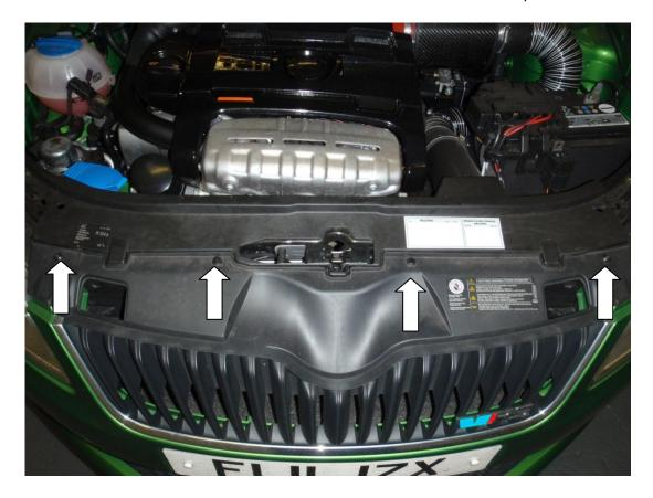
7. In the lower front grille there are two small grilles that need to be removed behind them are another two T30 torx screws, remove these.
