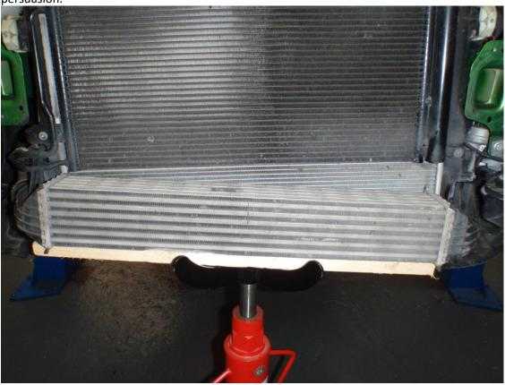
19. You can now fit your Forge intercooler in the same way you removed the stock one i.e. push the left side of the core up on to the radiator first.
