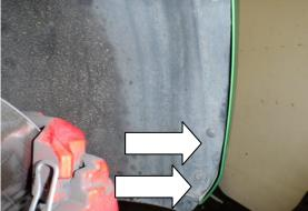
5. Once these Torx screws have been removed pull down the inner arch to reveal two more torx screws. You will need a Torx 25 with ratchet as these are a bit tricky to remove.
