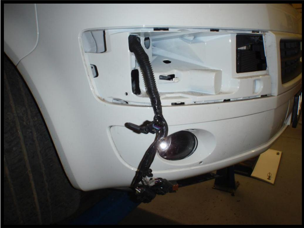
14. On the right side of the vehicle, unplug the connector from behind the headlight.
