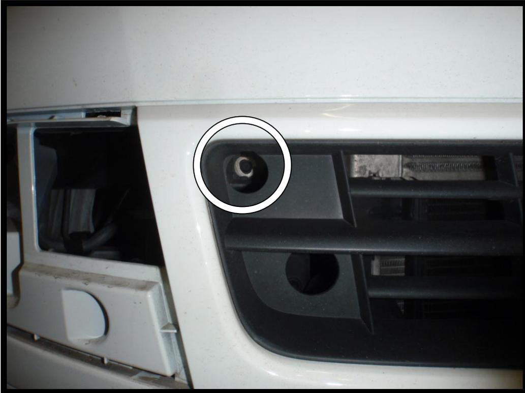
16. You will need to rest the bumper on some boxes or trestles, remove the front right light which allows clearance to remove the wiring. The bumper can now be completely removed.
