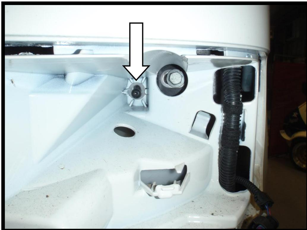
13. Pull out the wiring from the bottom and unclip it from the bumper on both sides.
